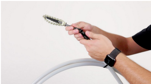
Snap on — line up the leader and push; the SpeedConnector locks it to the cable.
