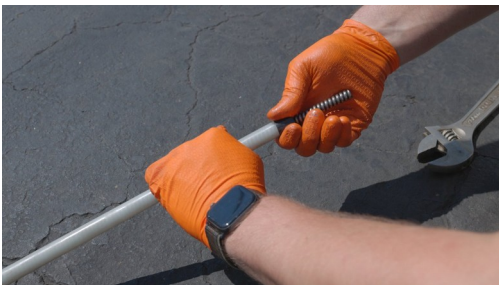
Start the cap clockwise by hand.
