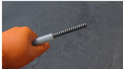
Trimmed 5"+ — cable exposed for direct chains.
