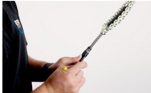
Disconnect — compress the button and pull the leader off.
