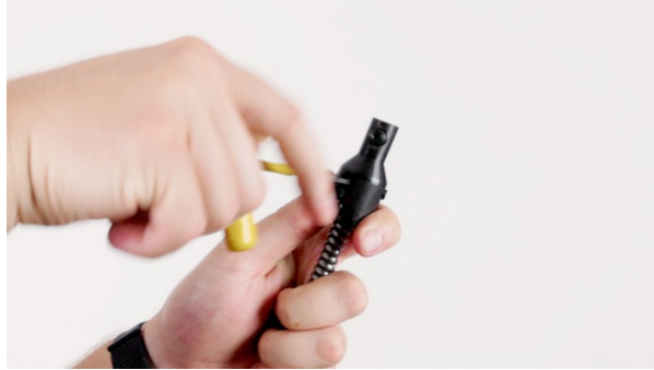
Place the set-screw connector on the cable and tighten the set screws with a 1/8" Allen key.
