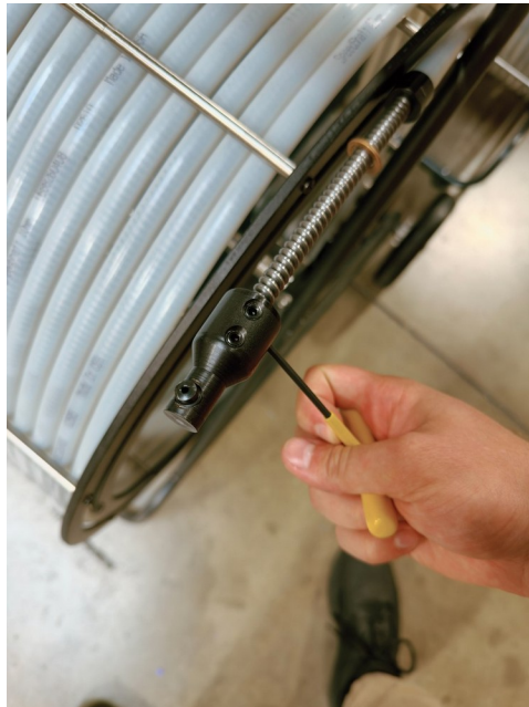
Take the SpeedConnector off with a 1/8" Allen key (if it's a crimp-on, cut it off with a grinder).
