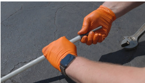
Start the cap clockwise by hand.
