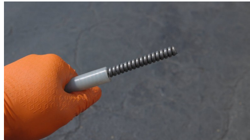
Trimmed 5"+ — cable exposed for direct chains.
