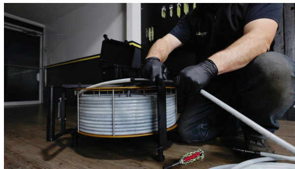
Add length — the SpeedConnector joins a SpeedShaft® extension cable to the machine the same way. Total recommended run on the SpeedCut® Mini+ Wheels: 125 ft (100 ft recommended).
