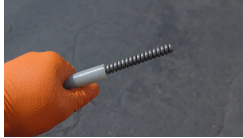
Trimmed 5"+ — cable exposed for direct chains.
